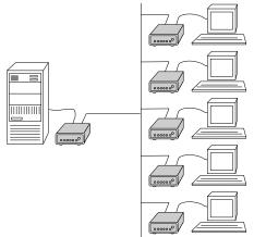
Figure 5. Typical multipoint set-up
